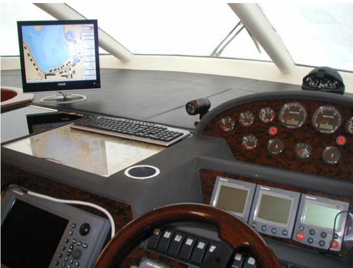
MY Princess 55, Murter, Brodski PC i NavPro, Internet, spojeni svi brodski instrumenti i autopilot na PC i NavPro
